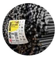
This EPD refers to construction products hot rolled structural steel bars and coils produced at Acciaierie di Sicilia plant placed in Catania (Italy), with electric arc furnace technology starting from post and pre consumer steel scraps. The homogeneous and repeatable mechanical features of steel guarantee excellent performance in any type of construction and geographical area, since they have high ductility.
